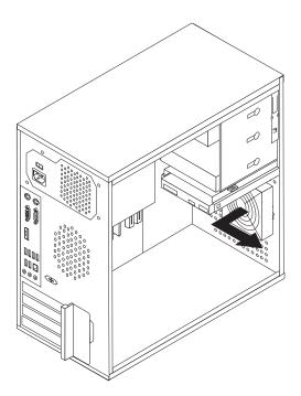
Figure 31. Removing the front fan assembly
